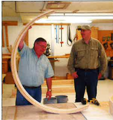
Louie Forseide (left) of GF Custom Woodwork, Inc. shows Greg West of Hepper Olson Architects a rebuilt part for the round windows for the front of the bank. Louie's company is working on replicating the windows and entrance which are scheduled for installation this fall.
